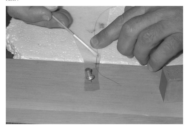
Here the first string is secured at the head, about 1/8 inch from the luff. The glue (described in the introduction) is applied with a Q-tip stuck on the end of a bamboo skewer. It gives better control than a brush. Only a half inch of string is stuck down at this point.
