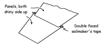
Therefore, the sail is made with the shiny surfaces of the panels facing all facing the same side of the sail. See **Figure 2**, compliments of Jeff Proulx.
