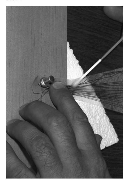
Here, three sets of five threads have already been applied from the head to the tack or clew of the sail. The last set of five is being stuck down at the head. (This sail will have 20 threads radiating from the head.) With practice, it's possible to glue two or three threads to the head at once, as shown here. The small foam block supports the sail as this is done.
