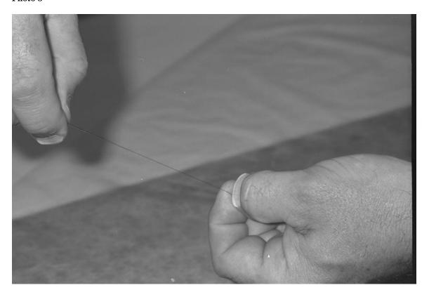
If you are using the Kevlar beading thread mentioned in the introduction (available from TSI, 1-800-426-9984) you will find that it has a natural curl as it comes off the spool. This can be largely removed by pulling the thread between your thumbnail and finger. (Be careful not to cut your finger by pulling too hard.)
