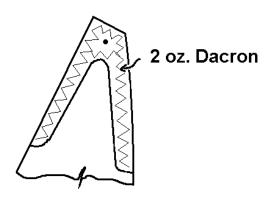
of overbend wrinkle which is formed from excessive loading. (I call these 'overload wrinkles'. You may also see them elsewhere on a highly loaded sail.) The path of the wrinkle will point to the region of overload.
