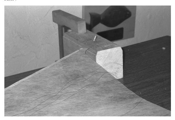
Photo 7 shows how the tack is supported, in this case for a jib. Note the luff pocket for the jibstay at the upper left. You can also see five strings draped along the sail, prior to their being glued in position. Support the clew in a similar manner.
