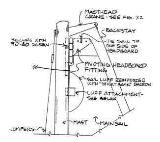
mast. Drill thorough the grommet and the hinge leaf while they are clamped together. Use a small drill bit (say 0.040 inches) to help keep the headboard in the proper place. (A large hole allows too much slop.)
