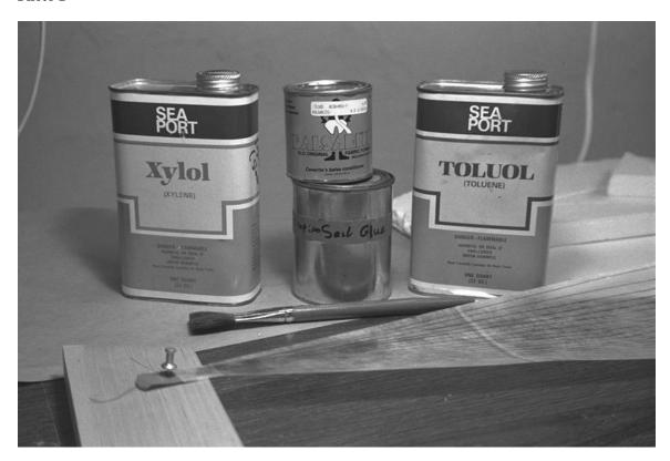
Some of the things that you will need are shown above. The most convenient work surface is your sail board. If you have not already made one, there is an article in the appendix on laying out the sail plan on the board. Here, a nearly finished sail is suspended above the board, pinned to blocks. There is more on this to follow. The strings are glued to the sail blank (shiny side to prevent curling) with thinned Balsarite. Use the original formula, No. 6000.
