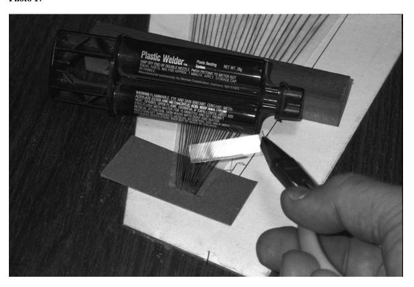
Now that all the threads are finally glued to the sail, the little tabs on the corners are cut off, leaving the sail at its final dimensions. At this point we need to evenly transfer the load on all the threads to the corner reinforcements. Here's how:
