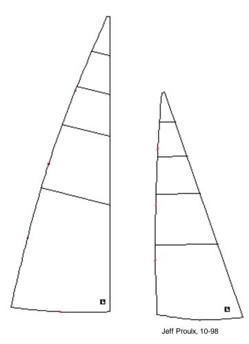
So knowing the actual amount of broadseaming is not required. It is predetermined by the block choice for that seam. (I did make an Excel worksheet that would compute the broadseam at each seam, but I didn't find any real use for it.)
