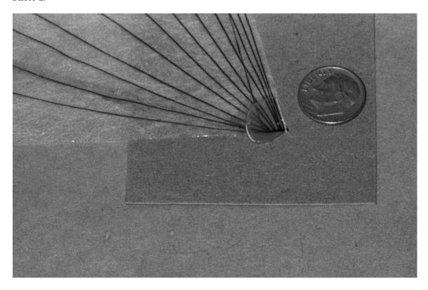
This photo shows the corner reinforcement at the tack of a jib. The tack of a main with a luff pocket would be made the same way. The sheet acetate reinforcement is attached in the same way as was done at the head. Although the small quarter circle of plastic has a radius of only about 3/8 inch, the result is amazingly strong. If done properly it's way in excess of working loads, as are the other corner attachments made this way.
