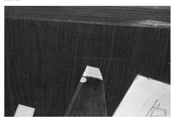
Once the sheet acetate is glued in place and trimmed, cover it with small pieces of 'stickyback' (sailmaker's patching and repair material). You could use spinnaker repair tape instead. Do not use *MonoKote* trim material, as it will come loose after several years.
